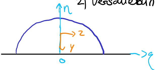
$$I_{z, \text{bez} \mid 0} = \iint_A n^2 dA = \int_0^{\pi} \int_0^R r^2 \sin^2 \phi \ r \ dr \ d\phi$$
