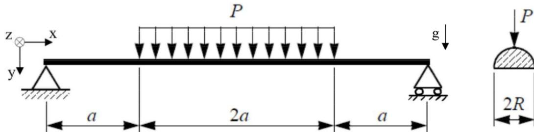
Geg:  $P = 5 \text{ kN}$ ,  $E = 210 \text{ GPa}$ ,  $a = 50 \text{ cm}$ ,  $\rho = 7,85 \frac{\text{kg}}{\text{dm}^3}$ ,  $g = 9,81 \frac{\text{m}}{\text{s}^2}$
