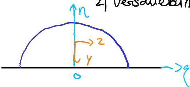
$$I_{z, \text{bezgl. } 0} = \iint_A n^2 dA = \int_0^{\pi} \int_0^R r^2 \sin^2 \varphi r dr d\varphi$$
