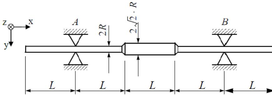
$$\text{Geg: } L = 1 \text{ m}, \sigma_{zul} = 20 \frac{\text{kN}}{\text{cm}^2}, f_G = 80 \frac{\text{N}}{\text{dm}^3}$$
