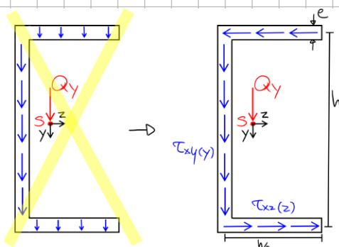
$$\tau_{xs}(s) = - \left( \frac{Q_y}{I_z} \right) \frac{1}{e(s)} \int_{\triangle A} y \, dA = - \left( \frac{Q_y}{I_z} \right) \frac{H_z(s)}{e(s)}$$
