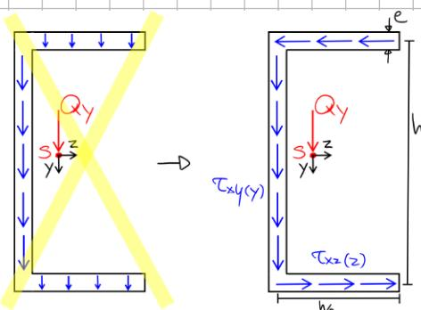
$$\tau_{xy}(s) = - \left( \frac{Q_y}{I_z} \right) \frac{1}{e(s)} \int_{\Delta A} y \, dA = - \left( \frac{Q_y}{I_z} \right) \frac{H_z(s)}{e(s)}$$
